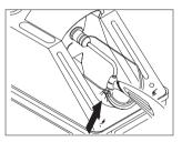
Press the instrument against the adaptor for about 10 seconds.
