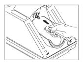
With its spray exit nozzle directed downwards, push the T1 adaptor onto the maintenance attachment. Initially, keep the cover open.
