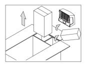
Take out the service oil, cleaning fluid, suction filter and the optional accessories from the side compartments.
