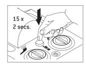
Press the program button about 15 times for 2 seconds with a pause of 2 seconds between each actuation.
