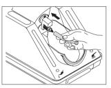
With its spray exit nozzle directed downwards, push the turbine with quick release coupling onto the adaptor until it engages.
