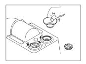
Unscrew the cap from the white storage container. Insert the white funnel.
