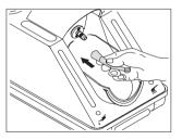
With its spray exit nozzle directed downwards, push the transmission instrument onto the maintenance attachment up to the limit stop. Close the cover and the waste disposal tray.
