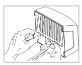
Press out the filter pack using a suitable implement.
