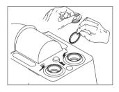
Unscrew the two caps and remove the two transport seals [malfunction!]!
