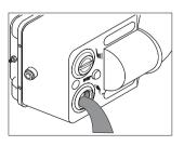
Empty the cleaning fluid and service oil from the storage containers. Do not empty the containers simultaneously. The cleaning fluid and service oil must not be mixed!
