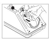
Press the green release button and pull off the turbine adaptor. Keep the adaptor in the recess.
