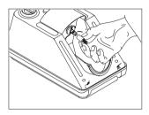
Pull the drip guard off the maintenance attachment and store it safely.
