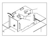
Remove the turbine adaptor. Lift out the Assistina in the fibreboard box.
