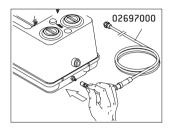
Push the quick release coupling of the connecting hose into the coupling socket on the Assistina. Connect the compressed air line using the 1/8« screw connection.
