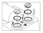
Fit a seal in each filler hole. Screw on the two caps. Before emptying the first container, fit the transport seal on the second container.
