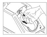
Fit the drip guard No. 02676400 on the maintenance attachment.
