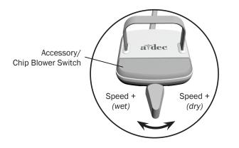
**NOTE** The lever foot control function can be reversed by a technician (change left direction to dry, right direction to wet). For more details, contact your authorized A-dec dealer.
