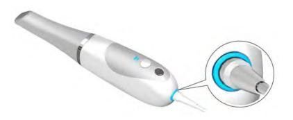
**Note:** The power indicator stops blinking and remains blue when the acquisition interface is open and the CS 3600 is ready to acquire images.
