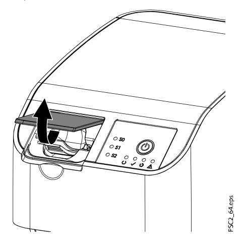
Place the light protection cover with the image plate centrally and straight onto the input unit. The torn-off side of the light protection cover faces down; the inactive (back) side of the image plate faces the operator.
