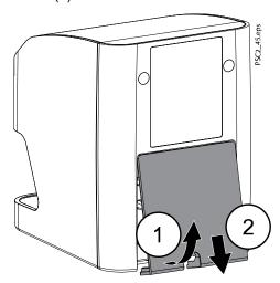
4. Plug in the connecting plug of the power supply unit into the socket connection of the device.
