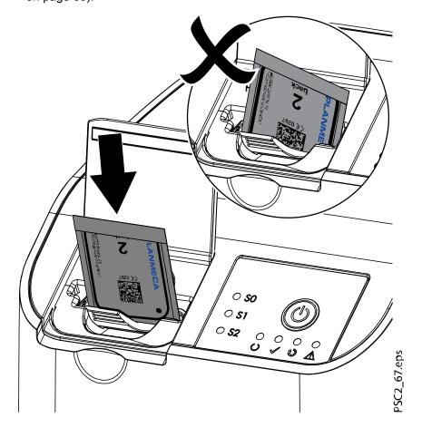
3. Slide the image plate out of the light protection cover downwards into the unit. The image plate must be inserted fully into the input unit.
