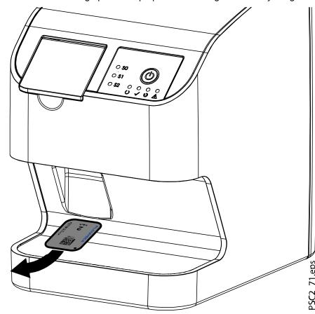
2. Remove the image plate and prepare it for taking a new X-ray image.
