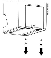
4. Pull the lower edge of the rear side cover out (1) and remove it downwards (2).
