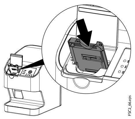
The green status LED lights up. The green display for the corresponding cartridge lights up. The input unit is ready.
