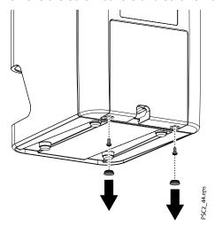
3. Pull the cover back (1) and remove downwards from the rear of the device (2).
