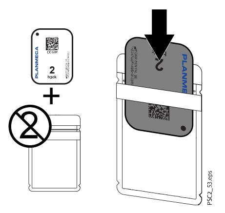
3. Pull off the adhesive strip (1), fold down the flap and close the light protection cover tightly by pressing together firmly (2).
