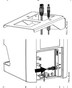
5. Lay the cables through the bracket and plug them into the unit.
