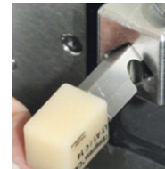
Block orientation: Vertical The notch points to the bottom right.
