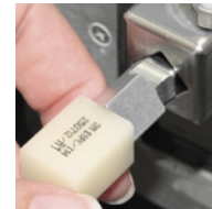
Block orientation: Horizontal The notch points to the top right.
