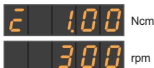
When the Endo function is switched on, the EasyPad display can be toggled between torque and speed to set the speed via the key *Display Mode / Clean*.
