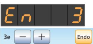
With the ultrasound handpiece removed: switching the endo mode on/off (limiting power)
