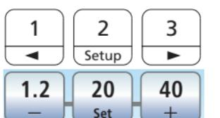
☞ The speed saved on the favorite key is shown in rpm (revolutions per minute). With the EasyTouch, the favorite key is highlighted orange.
