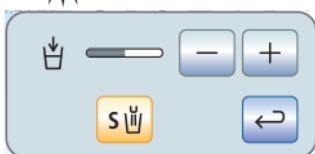
Pressing the *Tumbler filling* key (> 2 s) displays the setting text/program for coupling the tumbler filling to mouth rinsing position S and filling time.
