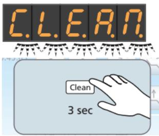
With instruments in place: switches the entire user interface of the dentist element to no function. The instruments of the dentist and assistant elements can no longer be activated. The Sivision monitor and the camera system are switched off. Pressing > 3 s again reactivates the treatment unit. This protects from interference from an external HF device and when cleaning the surface by ensuring that no functions can be accidentally triggered.
