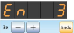
With the ultrasound handpiece removed: switching the endo mode on/off (limiting power)
