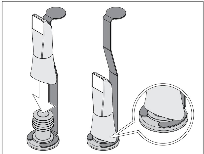
7. Press the sleeve onto the plug while holding the metal bracket firmly in place in order to ensure that no particle contamination or fluids penetrate the inside of the sleeve.
