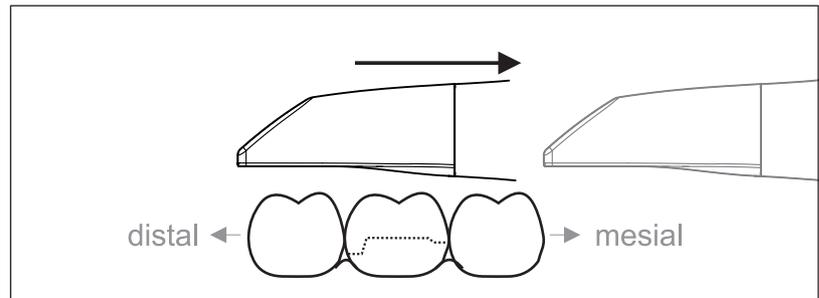
**Important:** Ensure that the distance between the coated sapphire glass of the scanner and the scanned surface is observed. The distance must be between 0-20 mm (ideally: 2mm). The scanner does not rest on the teeth or the gums.
