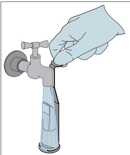
12. Carefully rinse the sleeve with tap water for at least 30 seconds while holding it with the bracket.
