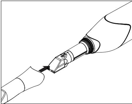
4. Place the white protective sleeve on the scanner head and place the scanner body in the scanner holder.
