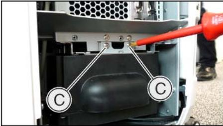
2. Slide in the storage battery using the guide rails and guide pins up to the stop and screw it in place with 2 fastening screws (C).
