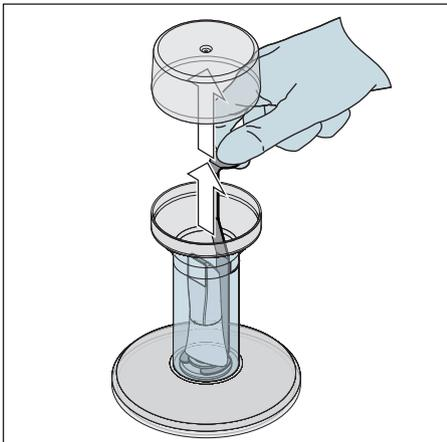
11. Remove the cover and take the bracket with the sleeve out of the container.
