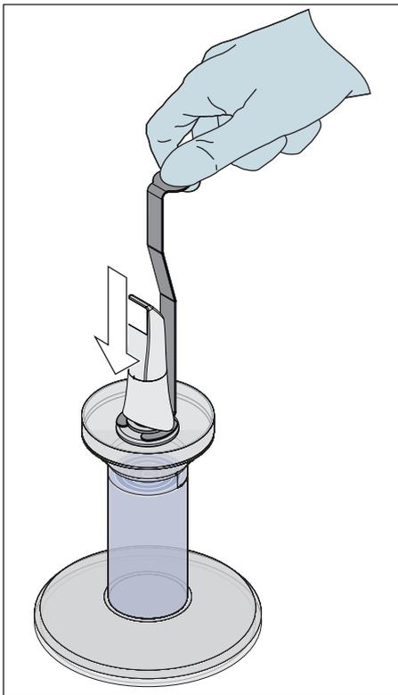
9. Insert the metal bracket with the sleeve.
