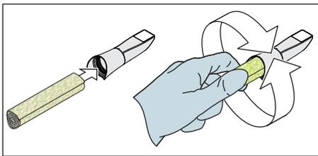
17. Dry the entire outer surface of the sleeve as well as the inner section around the plug using a soft lint-free cloth. Ensure that no fluid is able to penetrate the inside of the sleeve.
