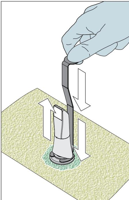
13. Remove the bracket from the sleeve carefully and slowly by pushing the bracket downwards. Ensure that the sleeve is pointing upwards so that no fluids are able to penetrate into the interior of the sleeve.
