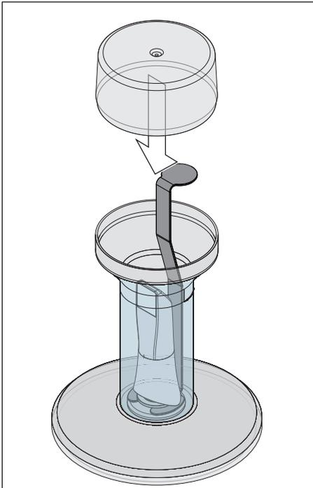
10. Place the cover on the container and leave the sleeve in the disinfectant for at least 12 minutes (CIDEX<sup>®</sup>OPA). The sleeve will not be damaged if it remains in the disinfectant for longer than the required time, but removing it shortly after the required time is recommended.
