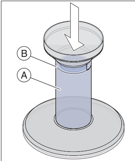
8. Carefully fill the HLD container up to the marking (B). You can use a funnel to pour in the fluid (A). Do not spill any disinfectant. Observe the safety instructions from the disinfectant manufacturer when cleaning if you do spill any disinfectant.
