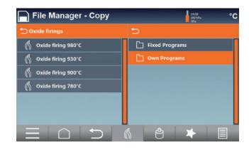
▶ Touch and hold <Oxide Firing 780 °C> in the left-hand window and drag it to the <Test Group> subgroup in the right-hand window.
